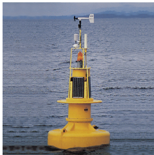
AIS fitted to a Tideland Signal SB-138P buoy complete with weather monitoring equipment during sea trials
